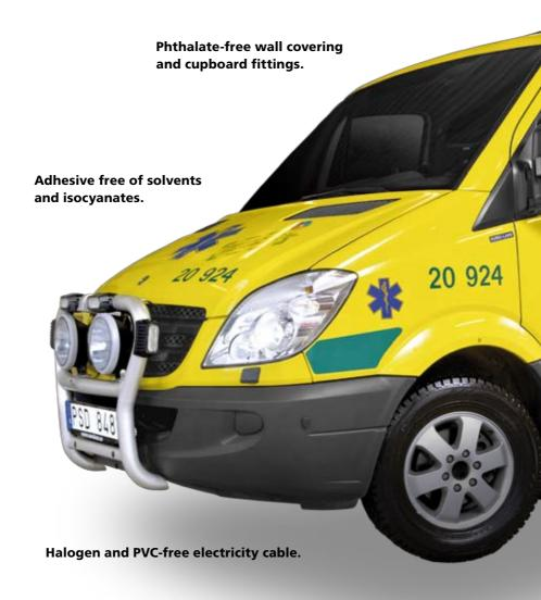
Aerodynamic alarm/light system with LEDs uses 5-10% less fuel. LEDs, Light Emitting Diodes, have low energy consumption and a long life span.
